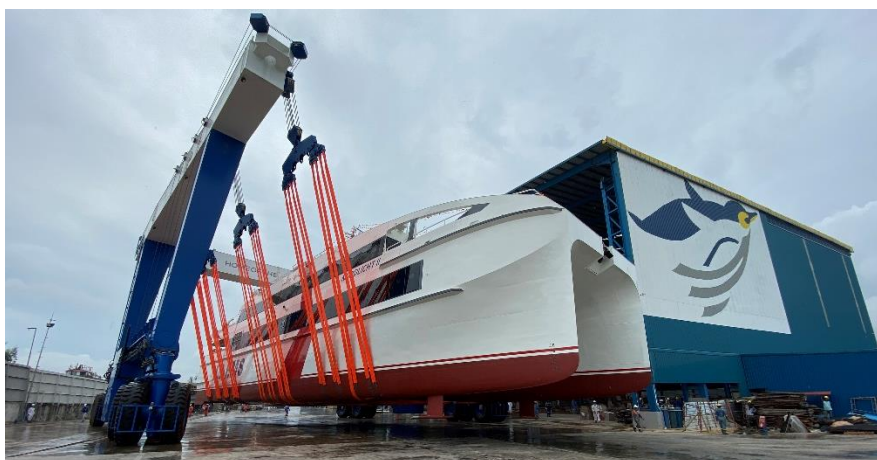
46m passenger ferry on the new straddle carrier
