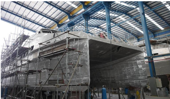
Passenger ferries under construction
