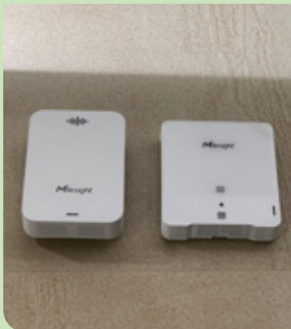
IAQ sensors to monitor air quality levels.
