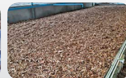
Eco-Innovation: Bio-filter system in Thai factories to minimise malodour
