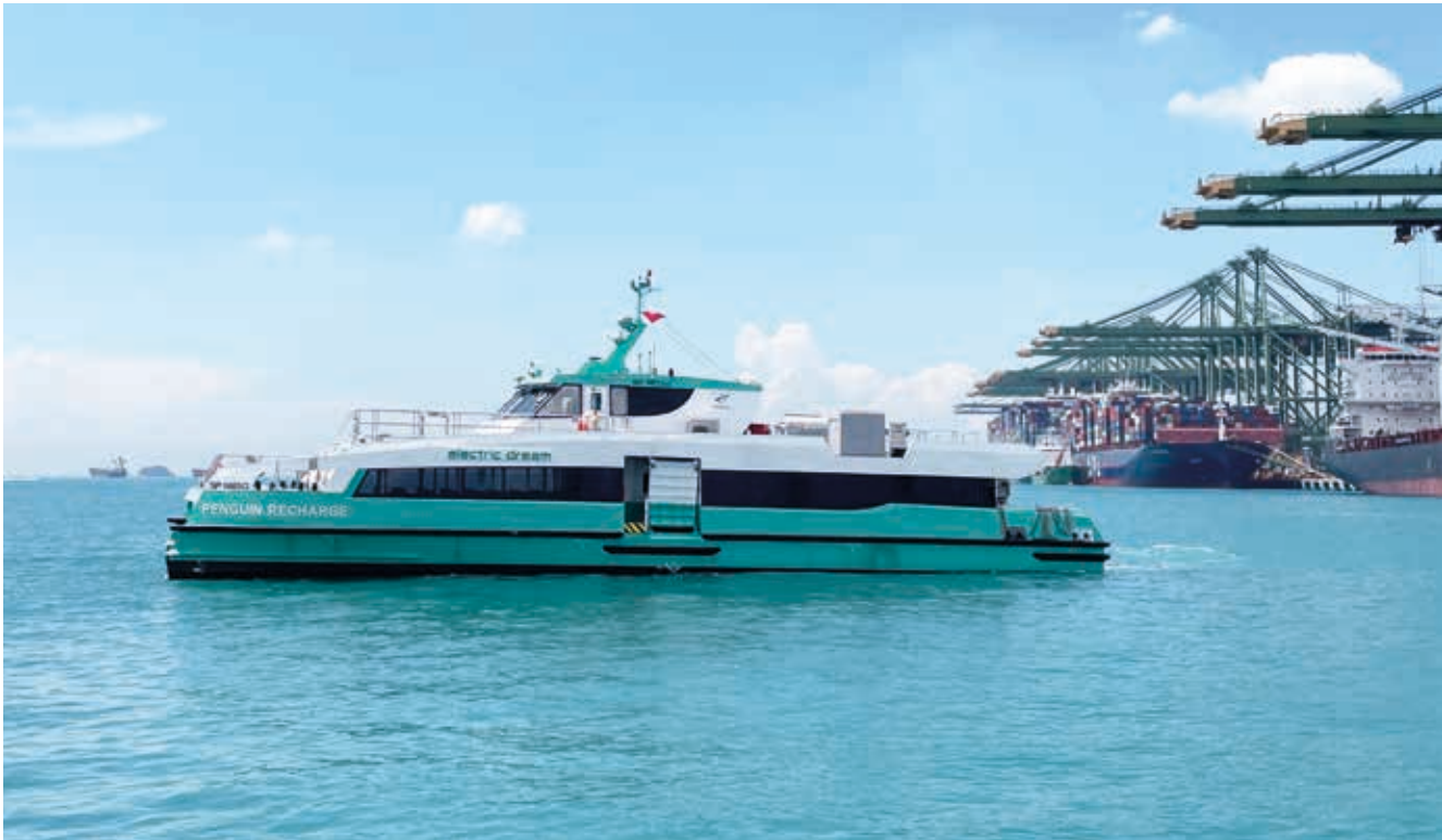
"Penguin Recharge": Cruising at 21 knots and recharging in less than 8 minutes.
