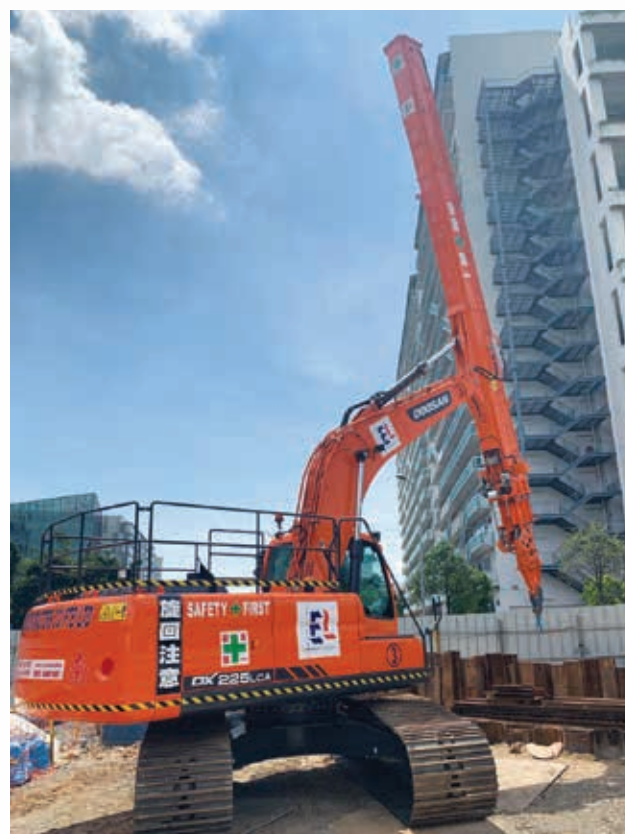
Newly purchased telescopic excavator to support OKP's existing and new projects.
