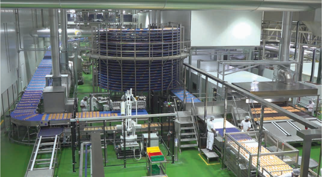
GBKL's new state-of-the-art roll and bun combination line.
