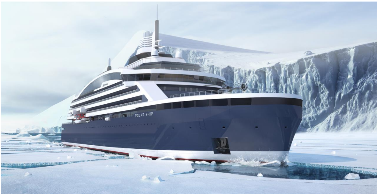
VARD 617 Electric hybrid cruise icebreaker with LNG propulsion Overall length: 150 m | Breadth: 28 m | Picture: Stirling Design International
