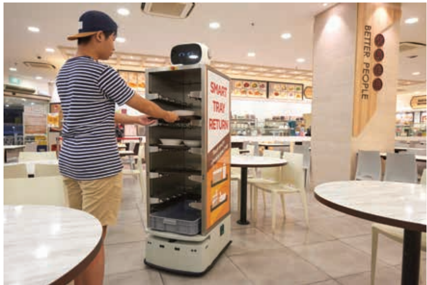
More than 40 of such smart tray return robots deployed to more than 16 of our food courts and coffee shop
