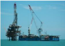
**TENDER RIG** is a barge moored alongside platform and contains crew quarters, mud tanks, mud pumps, and power generating systems. A tender rig carries its own drilling equipment and has a crane capable of erecting the derrick onto the neighboring platform.
