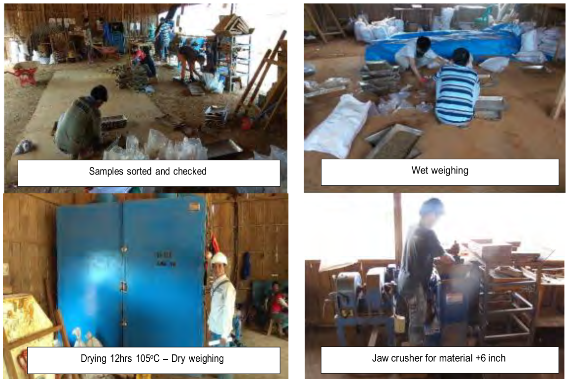
Figure 15.10 On Site Sample Preparation Facilities
