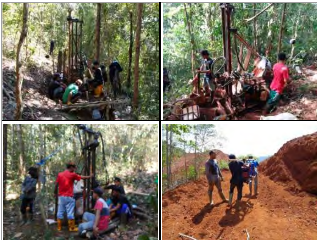
Figure 6.2 Drilling Activities using MD-175 Man-portable with Single Tube Core-barrel
