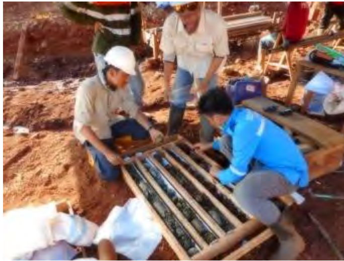
Figure 6.6 Core logging by field geologist on drilling site
