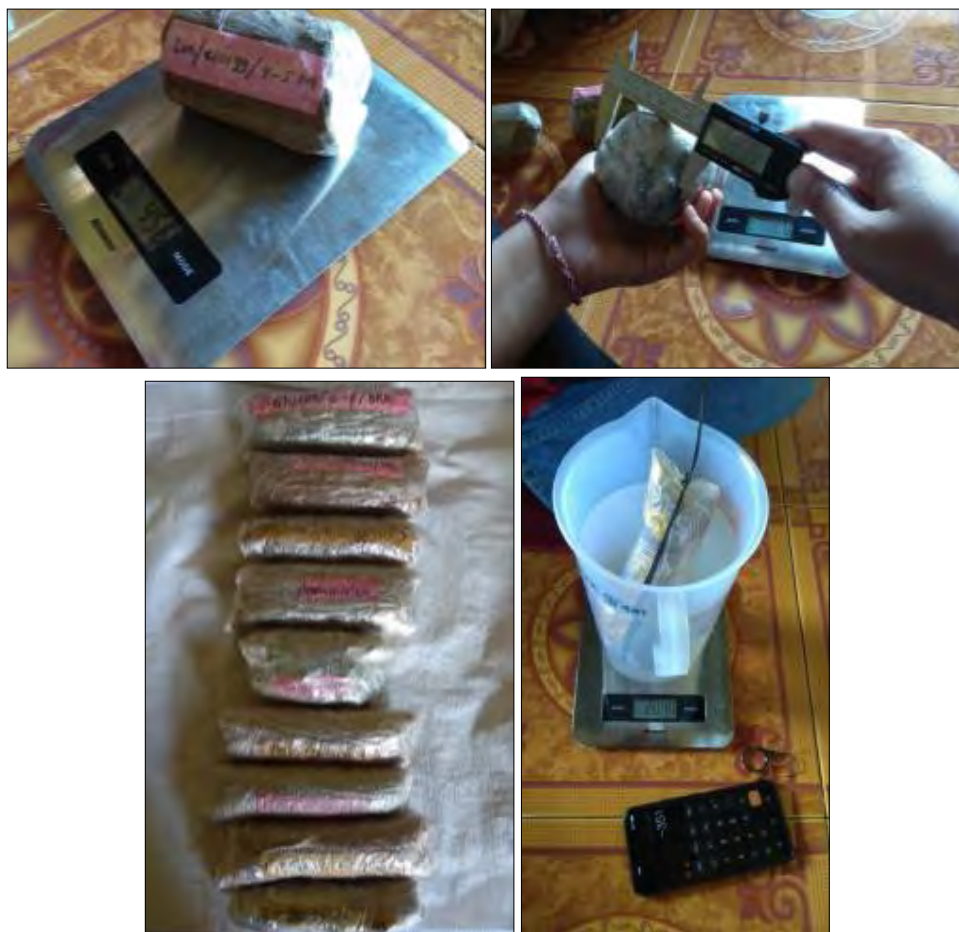
Figure 9.1 On-site core density measurement activities
