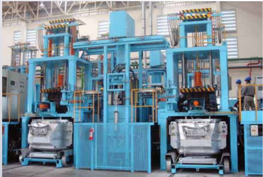
Low-pressure casting machines at the Stamford Sport Wheels Co Ltd production plant in Thailand.
