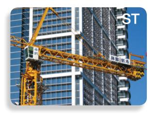
The ST towercranes are suitable for use in construction sites of all sizes. Introduced in 2000, the ST towercranes feature a conventional structural design where the tower head and tie bar reduces stress on the jib.
