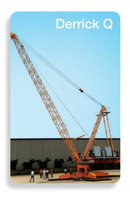
A towercrane under the Derrick Q series was successfully developed in 1998. The Derrick Q towercranes are designed for dismantling internal climbing towercranes in a safe and reliable manner. They are installed on the completed roof-tops of buildings and can be assembled and dismantled by hand.
