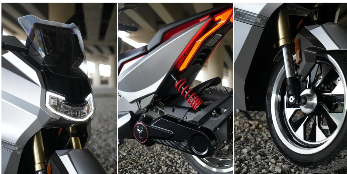
Unique vehicle design: Unibeam headlight & tail light, single aluminium swingarm, aluminium rim
