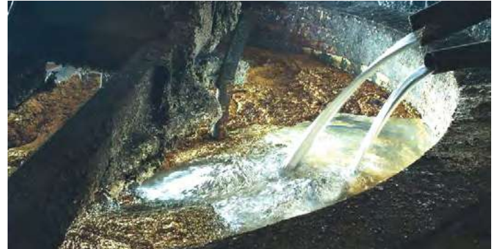
● Blending of molten tin in refinery kettle
