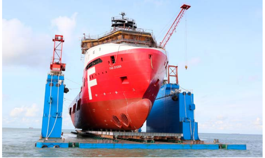
Far Sygna being launched by floating dock from Vard Vung Tau in Vietnam.
