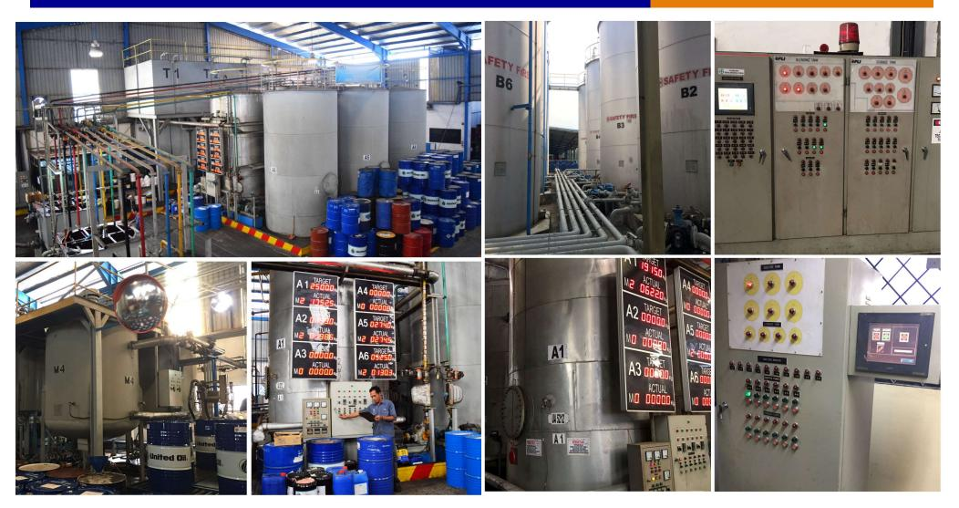
• 7 mixing tanks, and 6 additives tanks
