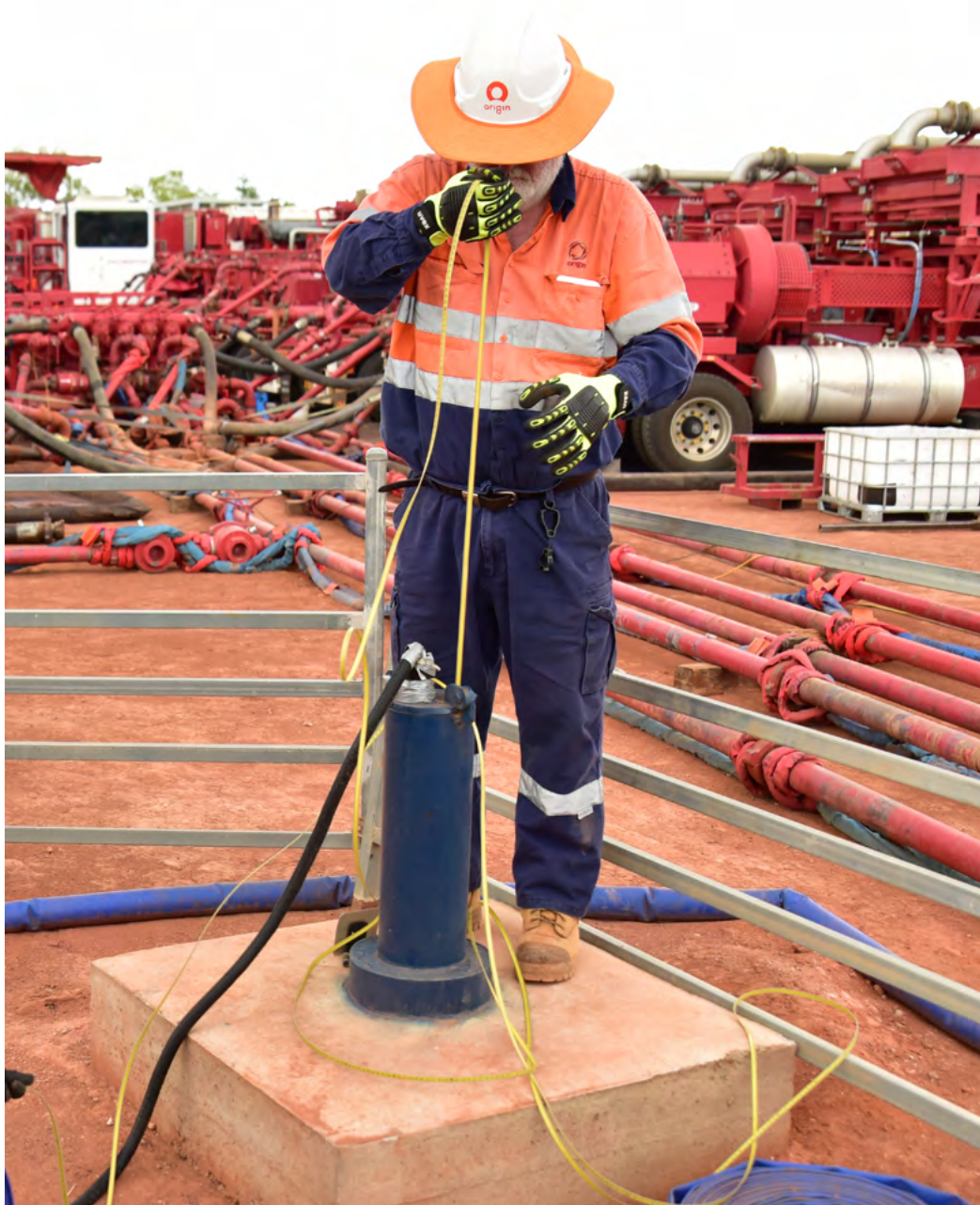
Continuous automated monitoring of groundwater during fracture stimulation at our Kyalla well site was verified by daily manual sampling of the two limestone aquifers in the area.
