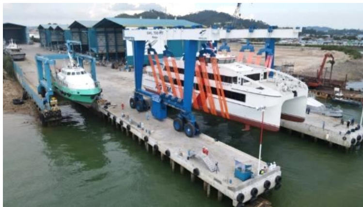
46m German ferry “Nordlicht II” was the first vessel to be launched by our new 700-ton marine travelift
