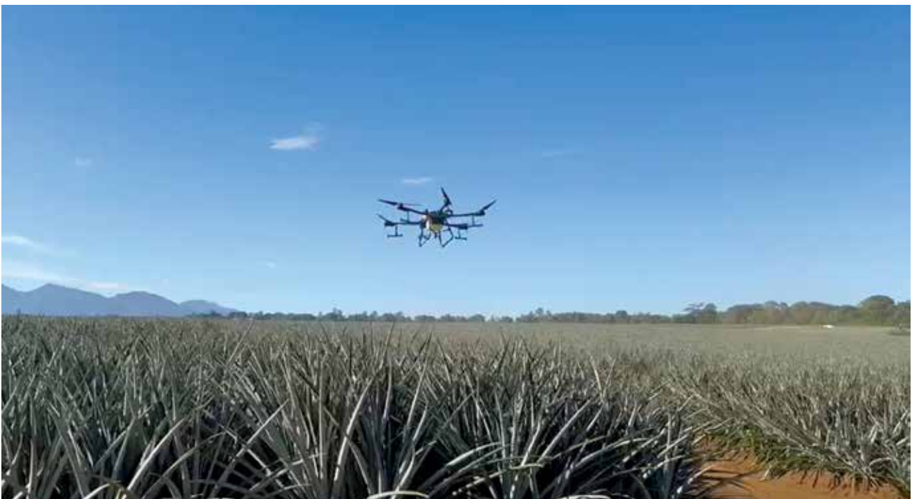
Unmanned Aerial Vehicles (drones) used in the plantation for foliar spray application and data gathering
