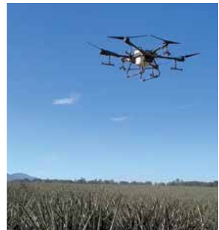
One of DMPI drones used in the plantation for monitoring plant health and mapping
