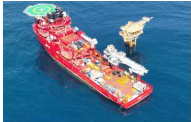
Figure 1.b : Picture showing Mermaid Van Gogh - Van Gogh comes with built-in saturation diving and air diving system, 120 beds, and a 150-ton crane.
