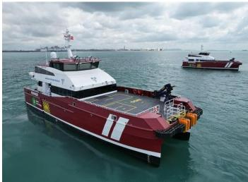
Hybrid-Electric Crew Transfer Vessels that meet IMO Tier III emission standards
