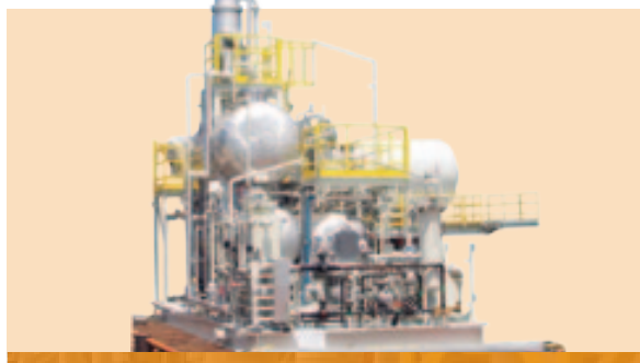
Glycol Dehydration Unit
