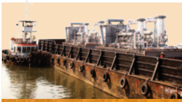
Flash Gas Compressor Package
