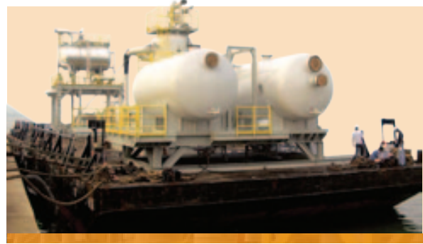
LP & HP Flare Scrubber Skid
