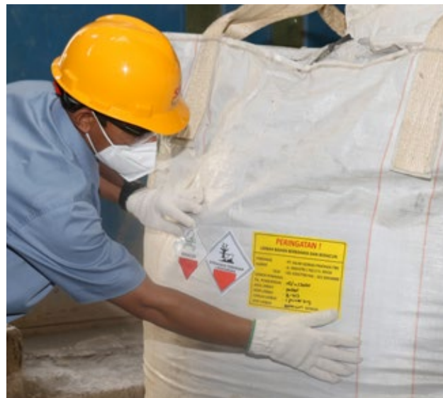
Preparing hazardous waste, such as spent bleaching earth for treatment at the Priok Refinery.
