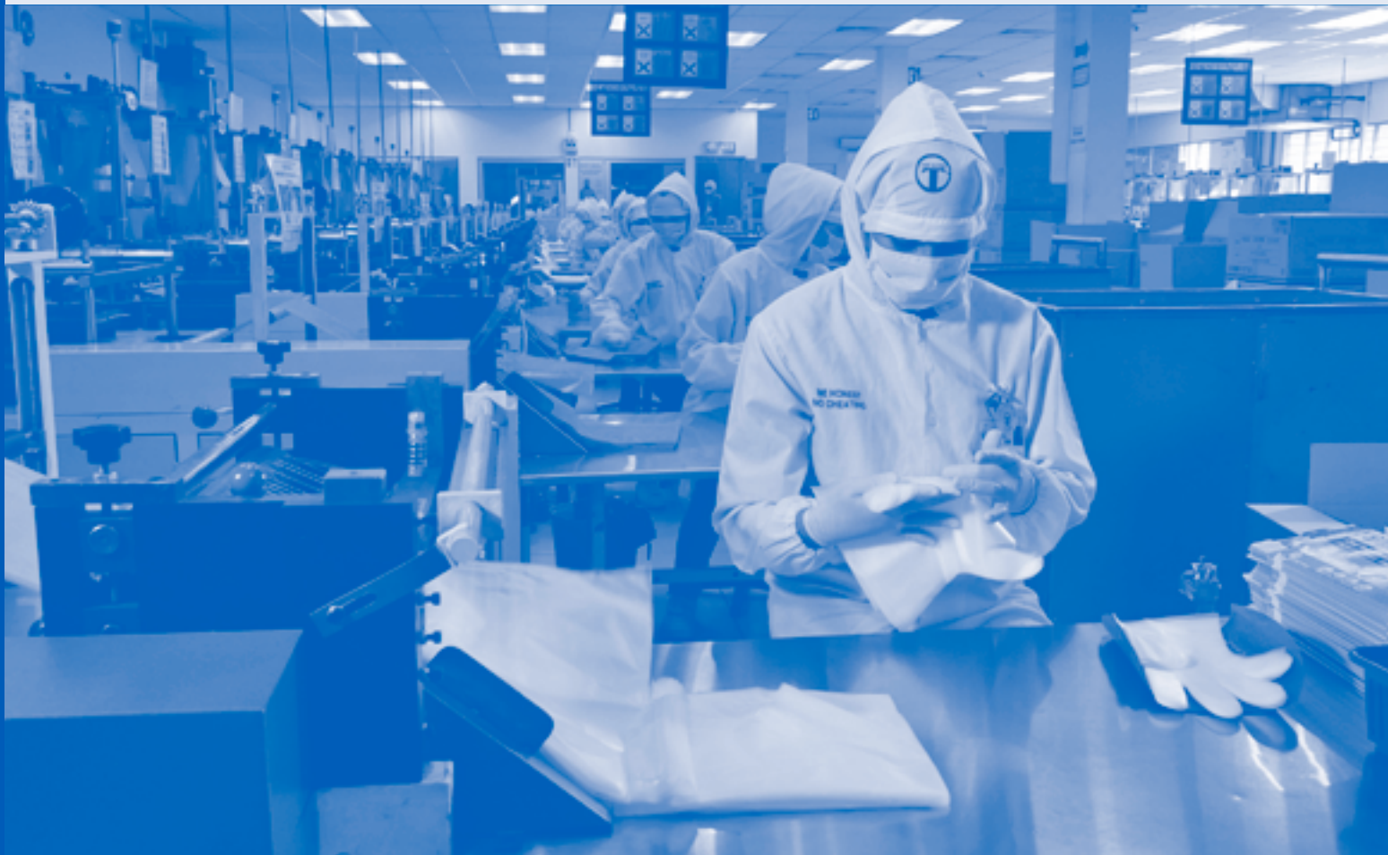
The stamping process in the production of Cast Polyethylene (CPE) gloves
