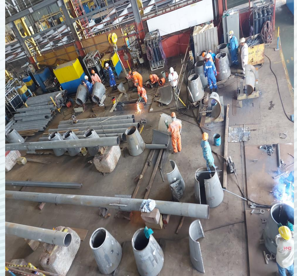
Fabrication and assembly of riser guard and antenna mast
