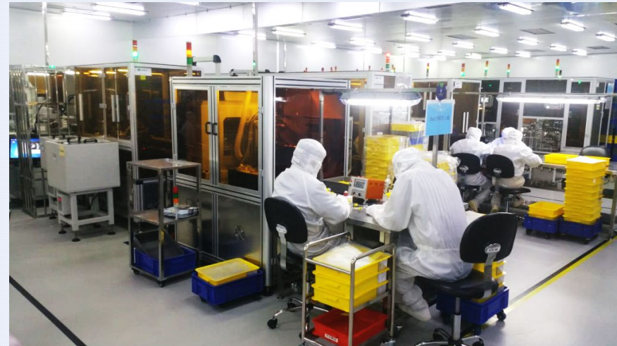
Assembly Automation Line in Class 7 (10k) Assembly Cleanroom
