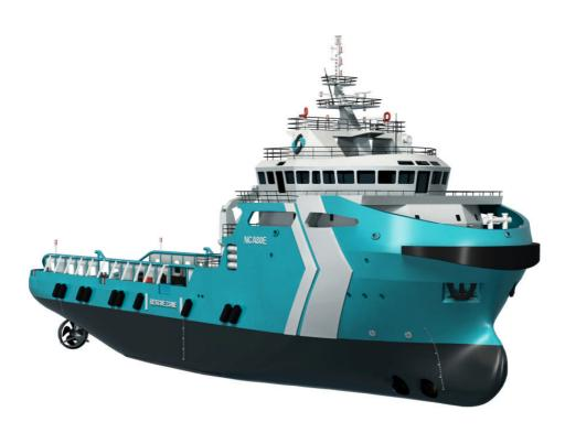
NCA80E, a 64.8m diesel electric powered AHTS with 80 tonnes bollard pull, based on Nam Cheong's proprietary design
