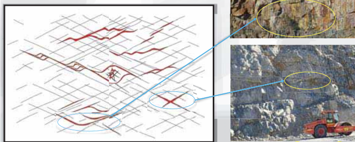
Figure 10. Fracture array architecture II (After Davis and Cowan 2017).
