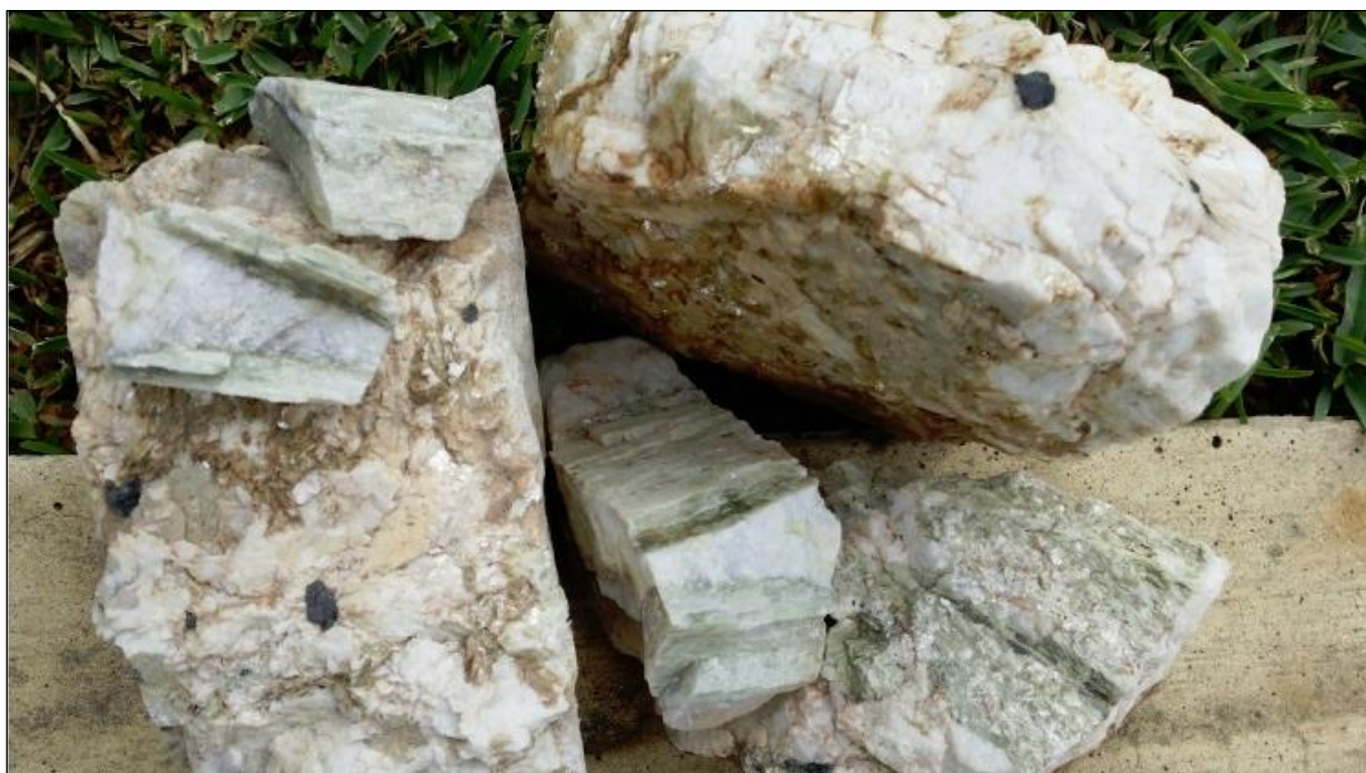
Figure 7: Pegmatite samples with tantalite and spodumene from Bald Hill
