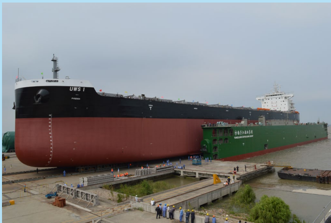
Moving the vessel onto the floating dock
