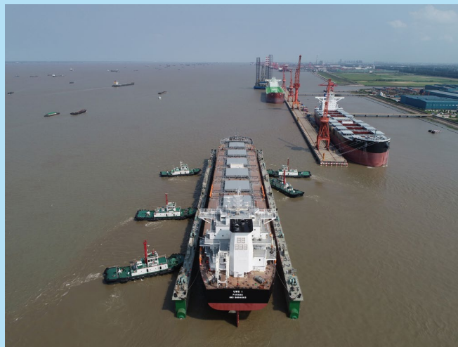
The floating dock submerges, the vessel is launched in the Yangtze River
