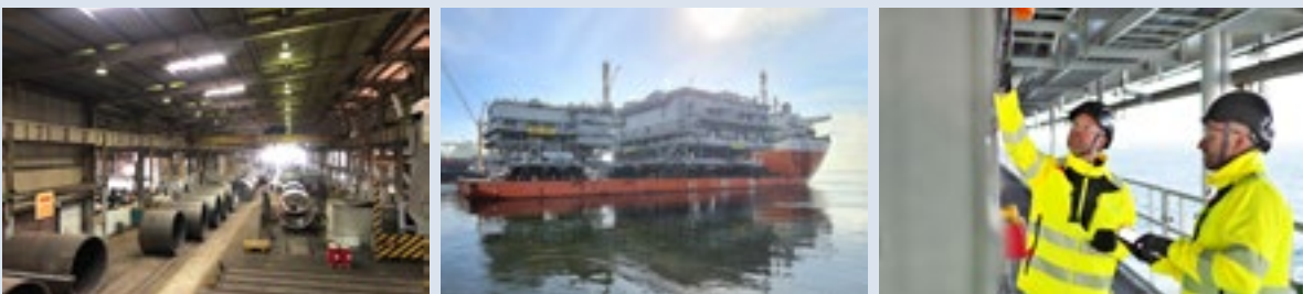
From left to right: Fabrication of typical jacket structure at our Batam Yard, Delivery of OSS and RCS topside from our Admiralty Yard and Planned preventive and maintenance service by ORS
