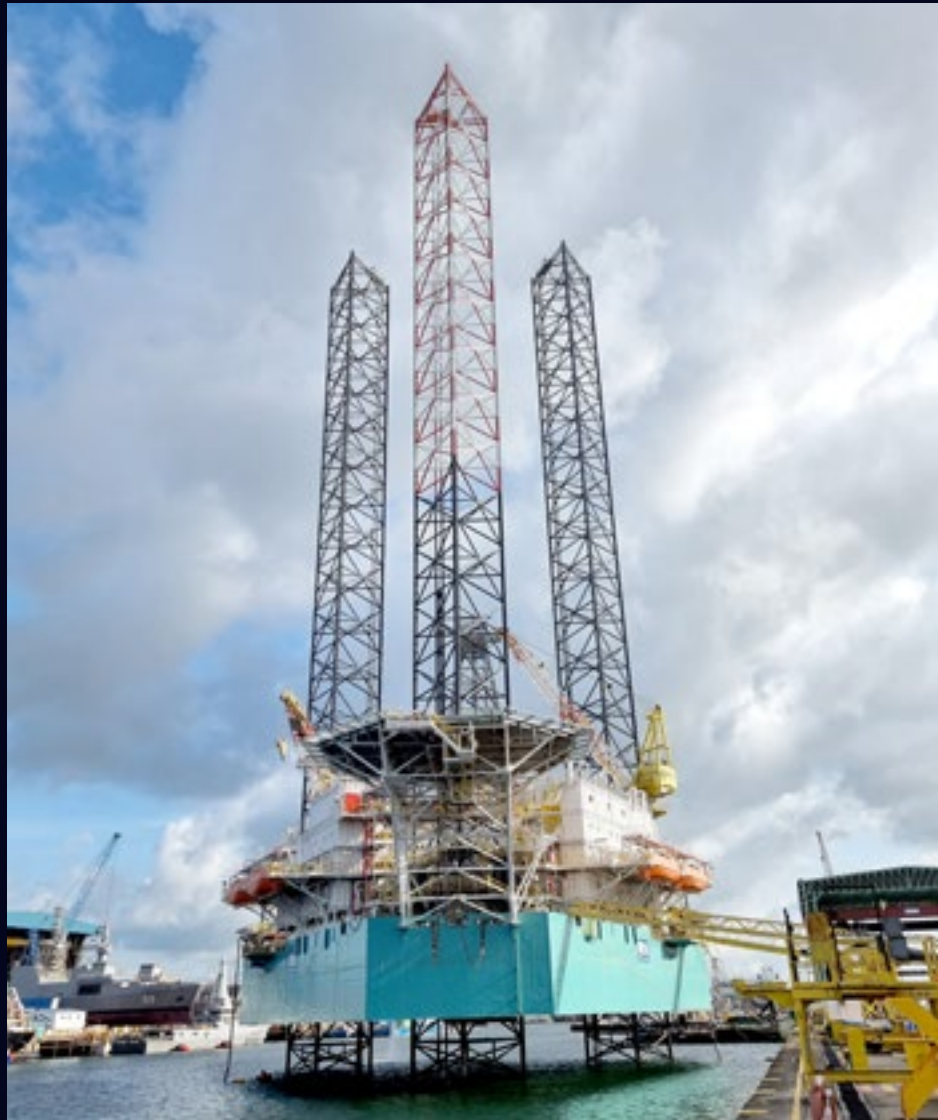
A pair of Jack-up rigs based on KFELS B class design, AISila and AISadiyat, delivered on schedule to ADNOC Drilling
