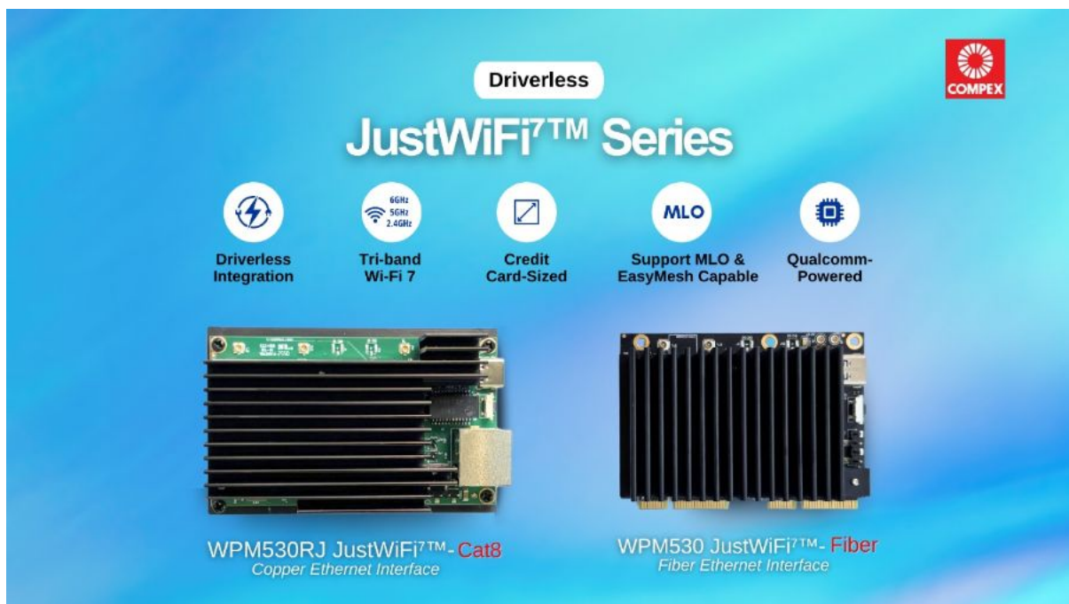
Figure 1 The driverless JustWiFi7™ Series enables simple, driver-free Wi-Fi 7 integration through SFP+ or 10Gbps RJ45 connectivity, reducing development effort and accelerating deployment.
