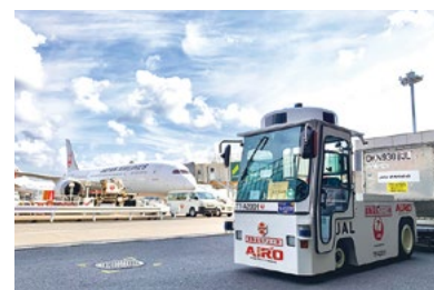
Self-driving towing tractor used in the airport Proof of Concept (PoC) test
