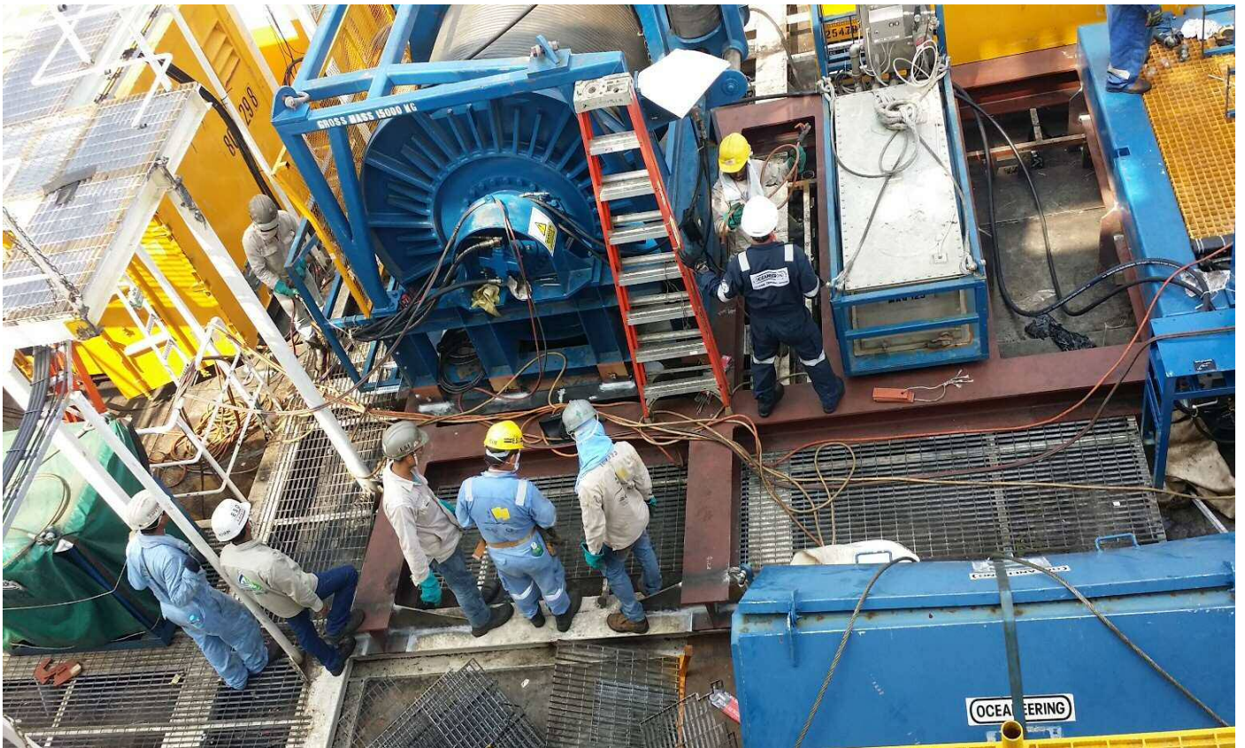
Above: Mobilisation of full Remotely Operated Vehicle (ROV) System.
