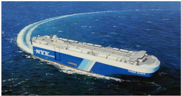
Name of vessel: m.v. Taurus Leader Capacity: 7,000 cars Built: Japan Flag: Singapore Length Overall: 199.98m Breadth: 35.80m Depth (Freeboard): 15.10m Gross Tonnage: 69,931
