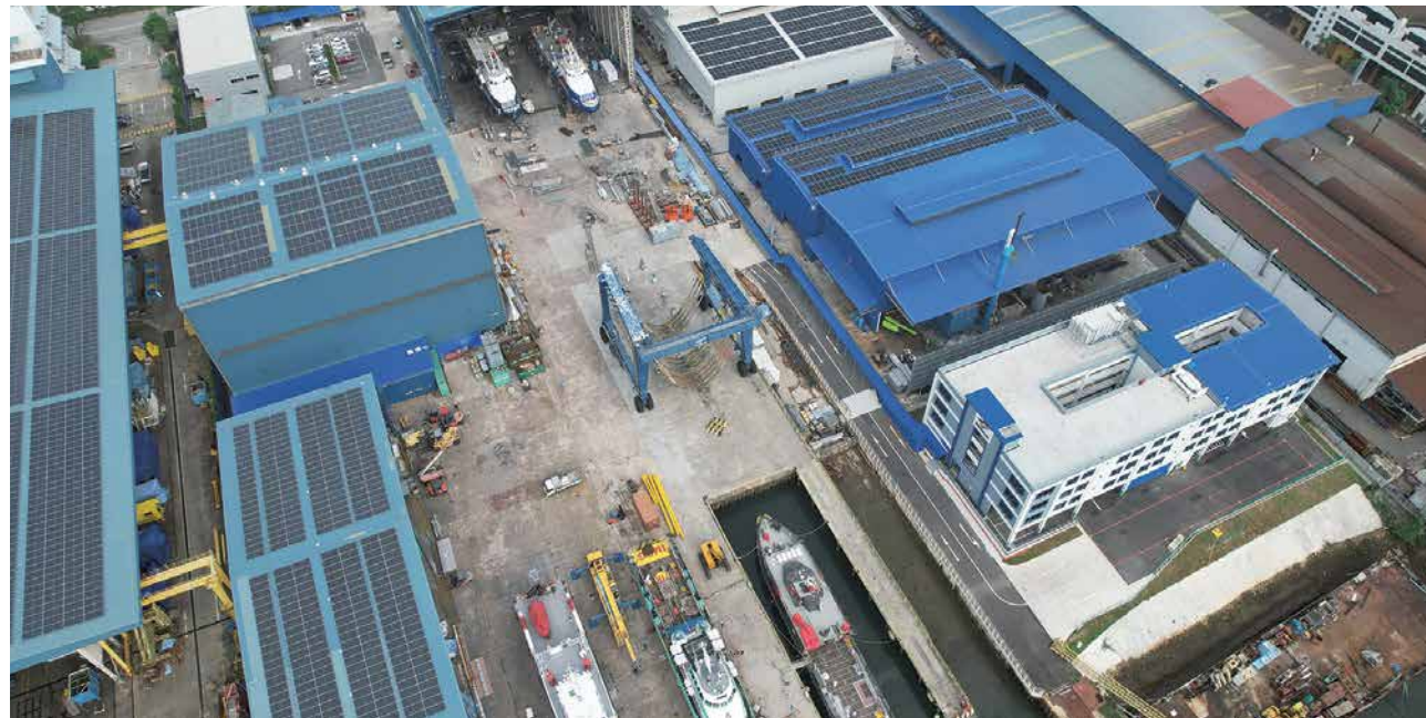
Penguin's 3-hectare shipyard and corporate headquarters in Tuas, fitted out with a solar array that supplies 80% of the yard's power requirements.
