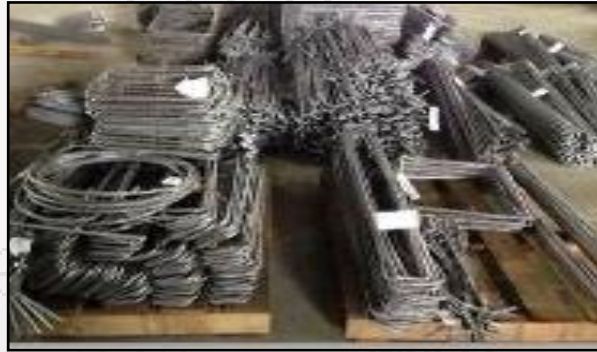
Rebar Cut and Bend
