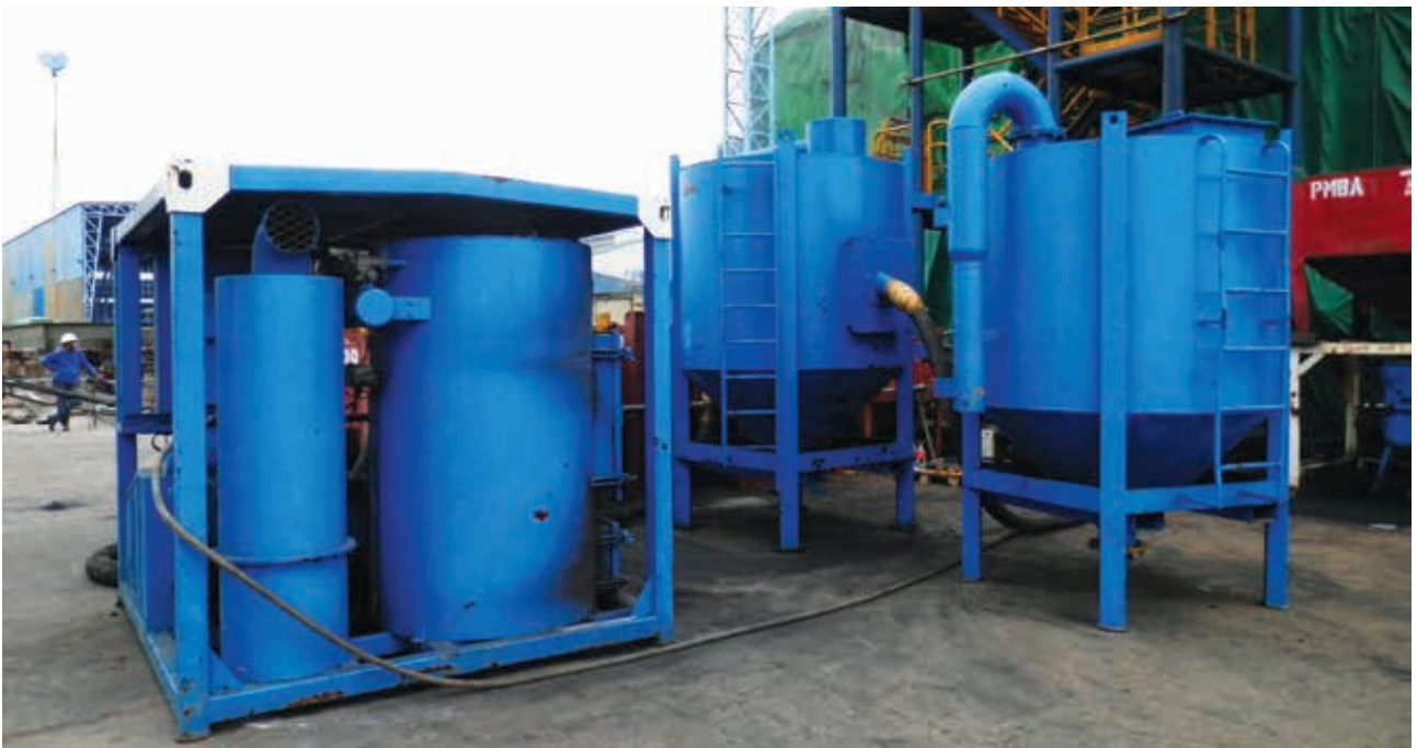
Vacuum pump for dust & grit extraction during blasting
