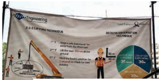
Safety signage: 30/30/30 Observation Technique (30 secs Observe your workplace, 30m Look at your surroundings, 30m Check above you)
