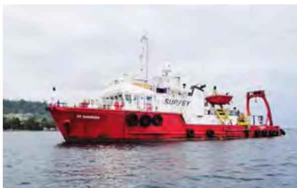
The SS '**Barakuda**' (formerly MV 'Mermaid Supporter') is a utility vessel equipped with an omni-directional bow thruster and accommodation for 30 personnel. This vessel has an extensive track record for performance of platform inspection and FPSO (Floating Production Storage and Offloading) facility underwater inspection projects in South-East Asia using a combination of ROV and surface diving methods. The SS 'Barakuda' is DNV classed and flies the Indonesian flag.
