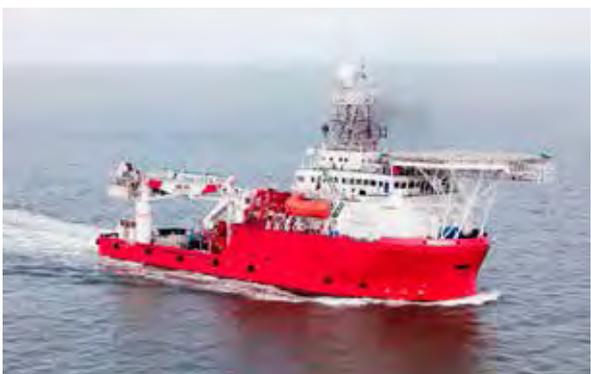
The DSV **'Windermere'** is a purpose-built DP2 diving support vessel. The vessel is chartered-in by Mermaid's Indonesian unit and has worldwide capabilities. The vessel is equipped with a built in 15-man saturation diving system complete with a self-propelled hyperbaric lifeboat. The vessel has a 50-tonne active heave-compensated subsea crane, a 40 tonne active heave-compensated crane and accommodation for 120 personnel. The DSV 'Windermere' is ABS classed and flies the Indonesian flag.
