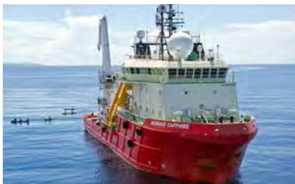
The RSV '**Mermaid Sapphire**' is a DP2 remotely operated vehicle ("ROV") support vessel equipped with a deepwater work-class ROV, a 23-tonne knuckle boom crane and accommodation for 60 personnel. In 2012, the vessel supported James Cameron in his historical deep sea dive to the Challenger Deep, the world's deepest point in the Pacific Ocean's Mariana Trench, 10.99km below ocean surface. The RSV 'Mermaid Sapphire' is ABS classed and flies the Panama flag.
