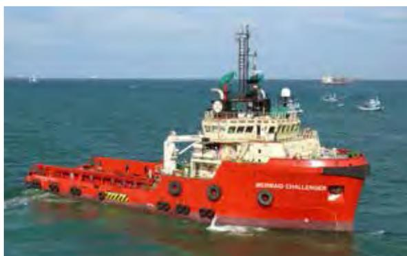
The MV '**Mermaid Challenger**' is a DP1 offshore support vessel with 72-tonne bollard-pull capacity, and is also suitable for performing ROV support vessel duties. This vessel can be equipped with heavy work-class ROVs and has accommodation for 38 personnel. Originally built as an anchor handling and tug supply vessel, the vessel has supported offshore operations in Vietnam for the past few years. The MV 'Mermaid Challenger' is DNV classed and flies the Panama flag.
