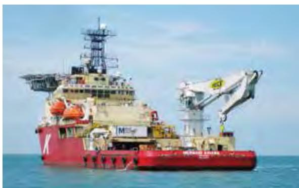
The DSV **'Mermaid Asiana'** is a purpose-built DP2 dive support and light construction vessel. The vessel is equipped with a built in 12-man single bell saturation diving system complete with a self-propelled hyperbaric lifeboat. The vessel also has a 100-tonne active heave-compensated knuckle boom crane and accommodation for 100 personnel. This vessel is designed for operations in the Middle East and Asia-Pacific region. The DSV 'Mermaid Asiana' is ABS classed and flies the Panama flag.
