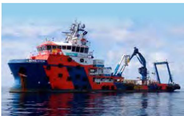
The RSV **'Resolution'** is a DP2 ROV and diving support vessel chartered-in by Mermaid's Indonesian unit. The vessel has been specially modified for IRM duties and construction support tasks and is also capable of geophysical and geotechnical survey. This vessel is equipped with a 20-tonne main crane, 3-tonne general purpose crane, 25-tonne A-frame and accommodation for 60 personnel. The RSV 'Resolution' is Bureau Veritas/BKI classed and flies the Indonesia flag.
