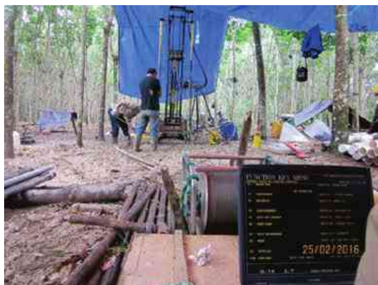
Figure 5:2 WRL Down-hole Geophysical Logging Operations
