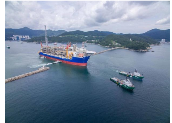
Towage and positioning of the INPEX-operated Ichthys Venturer FPSO facility
