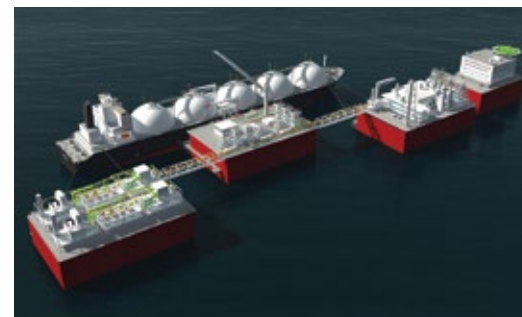
Gravifloat Modularised LNG and LPG terminals
