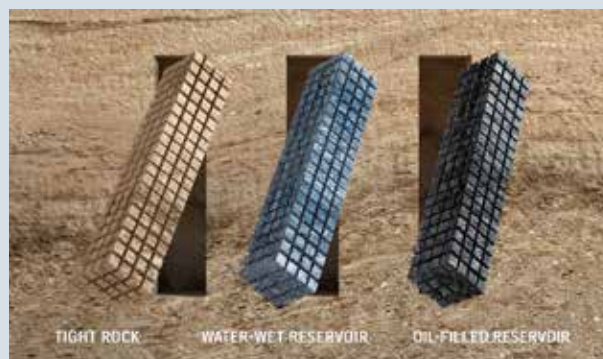
By analysing seismic resonance, the RVD results can identify liquid types and also separate tight rock from reservoirs with movable liquids.
