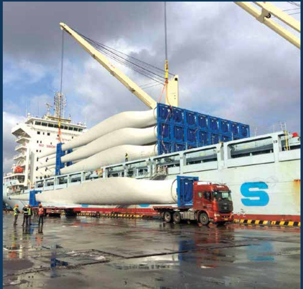
Loading windmill blades onto a vessel.
