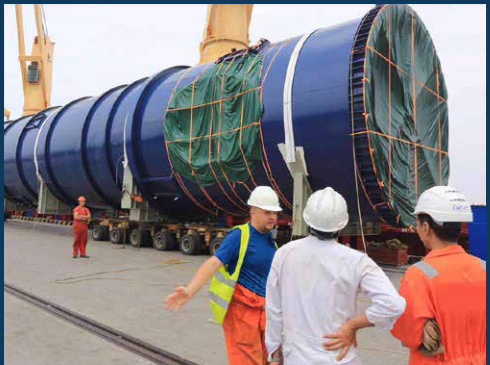
Hauling a cooling tower onboard.
