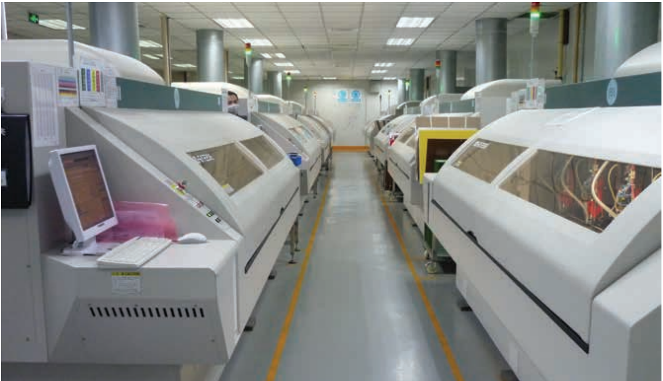
Rows of automated drilling machines humming their way to produce printed circuit boards at GulTech Jiangsu Plant, China.
