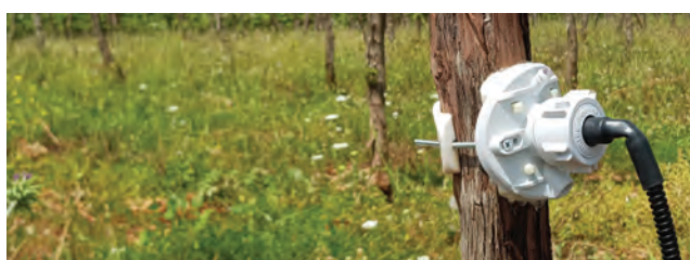
Saturas sensor installation in a vineyard
