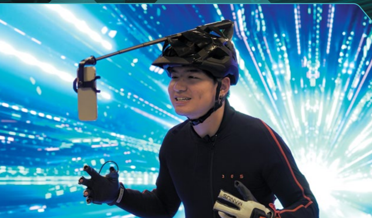
Motion Capture via sensor-embedded suit technology for precise real-time movement control that maps onto a virtual avatar
