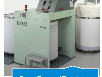
Draw Frame (Evenising and Parallelizing of fibre)
