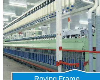
Roving Frame (Intermediate stage of Yarn forming)
