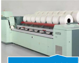
Comber (Removal of short fibre)
