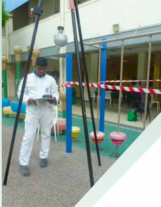
Impact attenuation test to measure a playground surface's shock absorbing properties to ensure it is within the safety guidelines.
