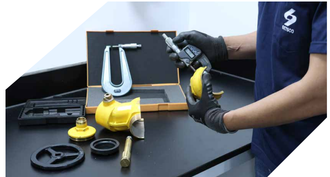
Evaluation of the dry riser landing valve's dimensional consistency and structural integrity.
